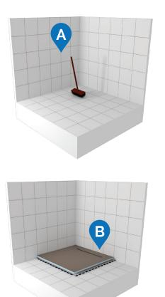
Prepare floor and walls and clean it from dust, debris. Remove garbage and make sure you have sufficient space for comfortable work. Prepare materials and tools necessary to complete the installation, you will probably need a level, chisel & hammer or jackhammer, pencil,measuring tape, brush, notched trowel, tile adhesive. Handsaw can be used to trim the shower tray to trim to size, but equal distances from both sides should be cut to preserve proper fall towards the drain.
