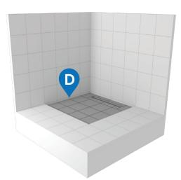
Find the best possible drain position and angle to connect it to your pipe work. Siphon trap can be rotated in 360° and waste pipe's height can be adjusted, giving much flexibility for proper positioning. Ensure the siphon trap is supported below with concrete. If created hole is too deep build up support with cement.
