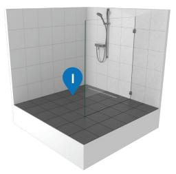
Distance from the shower tray surface to the top edge of vertical drain frame is 15 mm, so if you need to build up that space, use tile backer boards. They are perfect material to tile over and should be used as well over the rest of the floor. Wateproof the connections between boards and also floor/wall connections using tanking liquid and waterproof tape contained in waterproofing kit. Apply sealing corners and pipe collars where necessary. Liquid foil can be used as adhesive to stick these.
