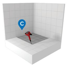
Remove existing concrete layer as thick as Showerlay using a chisel and hammer or jackhammer. Grind a square or rectangle matching previously drawed Showerlay shape. Identify future position of waste approximately 65 mm below the concrete surface and pipework.
