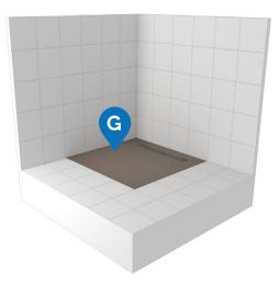
G Put the Showerlay down to check if it sits in correct position and if it's flushed with rest of the floor. Check if you are able to connect the siphon upper part with waste trap underneath the shower tray and if it sits on previously prepared support. Use the level to check if the tray is even and if the drain channel is the lowest place in the shower area. Test if the linear drain channel matches the hole in ply support.
